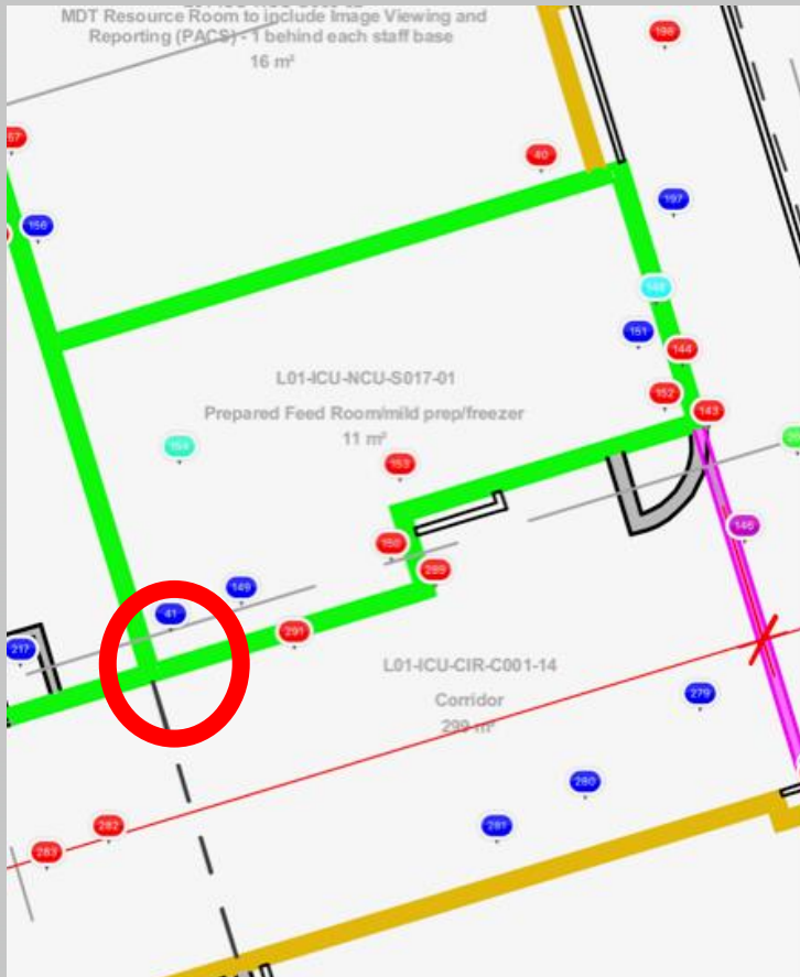
Example of a typical inspection issue identified. Take Tag 41 highlighted – firestopping damaged
